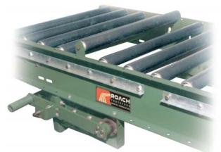
Manual operated power conveyor stops are hand operated and used where line control is required such as accumulation, indexing, inspection stations, etc. This stop is normally used on variable pressure accumulators and live roller conveyors.
