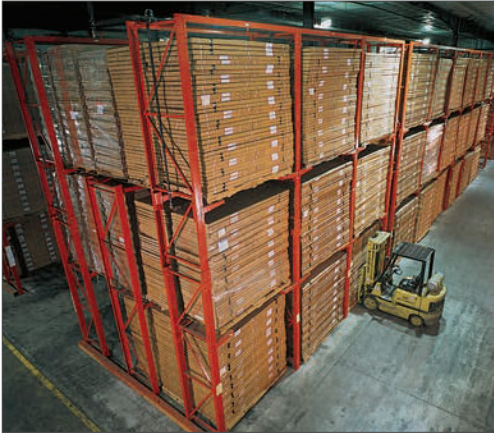
MECO OMAHA Drive-in Rack installation. Custom-designed for high density storage and efficient handling.
