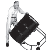
Push drum back on stand and grasp top and bottom chime
