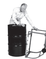
Tilt drum and slide Rock-It nose under chime
